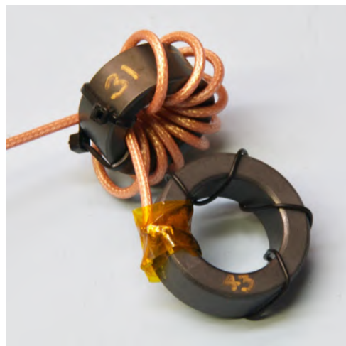
Figure 3. Wideband current transformer and common-mode choke. The 50-ohm terminating resistor is covered by tape.
